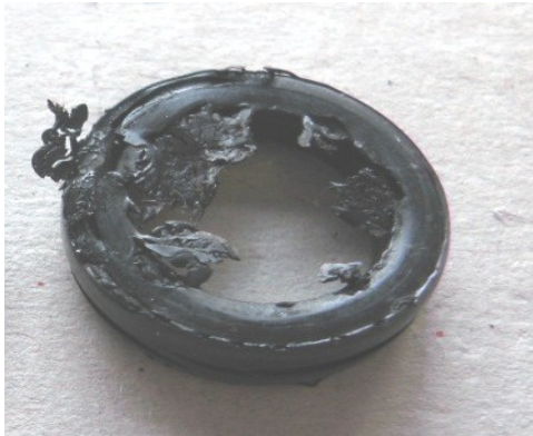
Figure 2 - ETP extrusion during rapid gas decompression following super critical CO 2 immersion.
