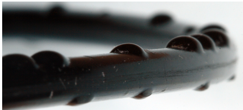
Figure 3 - Blister damage during rapid gas decompression following super critical CO 2 immersion.
