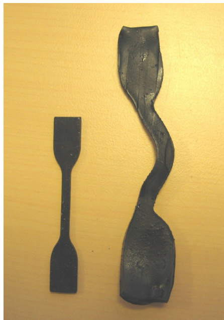
Figure 1 - steam swell comparison of HNBR dumbbell shown with un-aged dumbbell.
